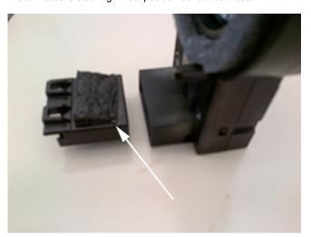
2. Add a piece of Adhesive Back Shim Stock the width of the connector to the flat surface on the male connector. This provides support to the connector
