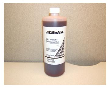
The transmission requires AW-1 Transmission Fluid, United States P/N 19256039 and in Canada P/N 19256040. **DO NOT** use DEXRON<sup>™</sup> - VI Automatic Transmission fluid as it is not compatible.
