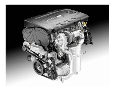
The 2.0L turbo-diesel engine provides greater fuel economy than a comparably sized gasoline engine through greater thermal efficiency, a higher compression ratio and an unthrottled combustion process. It features an iron cylinder block and a forged steel crankshaft, each designed to stand up to the greater cylinder pressures commensurate with a turbo-diesel engine.
