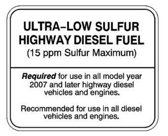
Caution: Use of diesel fuel other than Ultra Low Sulfur Diesel (15 ppm sulfur maximum) will cause damage to the exhaust after-treatment system. This damage would not be covered by the vehicle warranty. DO NOT use marine, locomotive, or boiler distillate fuel since it may contain higher sulfur levels.
