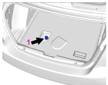
In the rear compartment of the vehicle, under the load floor is the DEF tank (1). The capacity of the tank is 4.9 gallons (18.5 L). This is enough DEF to provide a range of at least 10,000 miles (16,000 km) of driving between refills. The system is also designed for servicing to coincide with oil changes, for greater convenience.
