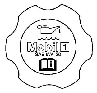
The following Corvette engines built at Wixom, Michigan are equipped with an OEM oil fill cap that identifies Mobil 1<sup>™</sup>, SAE 5W-30 as the engine oil that is required to be used in these engines.
