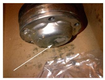
2. The front CV joint has a vent in the center of the cap that may expel grease if the propeller shaft is heavily compressed at the front CV joint during service. This grease expulsion under these conditions is normal and does not cause any significant loss to the joint.
