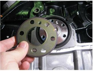
The reluctor wheel is located between the flywheel and the crankshaft. Once the flywheel is removed, the reluctor wheel can be transferred to the rear of the
