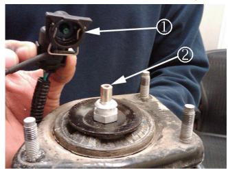
2. Disconnect the electrical connector (1) from the top of the applicable shock absorber (actuator) contact (2).
