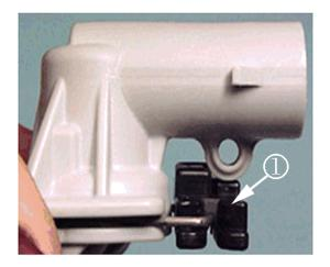
CTS Models built after February 22, 2011 have a CPA tab (1) as shown above as part of the connector. Vehicles built with this design should be less susceptible to being unseated. The CTS is the only vehicle to adopt this design change. All other products continue with the original style connector.
