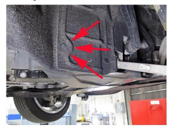
This condition may be caused by the tire contacting a raised section of the front wheelhouse splash shield.
