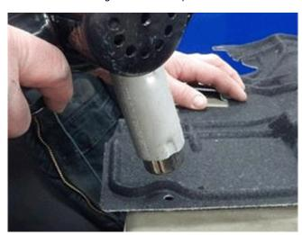
3. Heat the wheelhouse splash shield in a localized area to soften the part for approximately 1 minute (holding 1-2 inches above the part).
