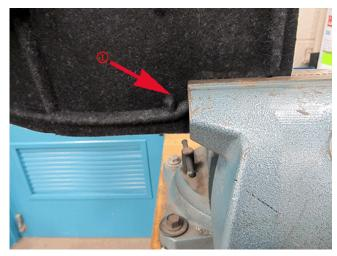
Using a bench vise, insert the splash shield as shown and close the jaws on the vise.Do not go past the rib (1) when inserting the splash shield into the vise. Allow the part to cool in the vise for a few minutes.
