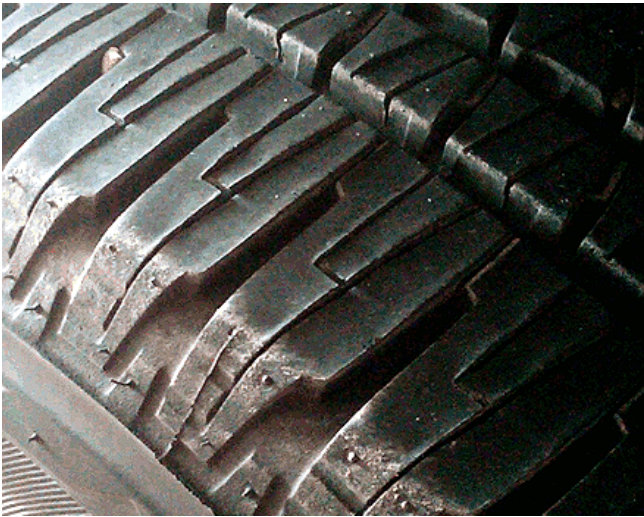
Figure 4: Detail Side View of Tire Shoulder Area - "NORMAL" Tire "Feathering" Wear
