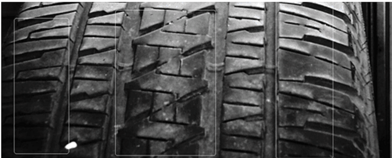
Figure 1: Full Tread View – “NORMAL” Tire “Feathering” Wear on the Shoulder/Adjacent/Center Ribs
