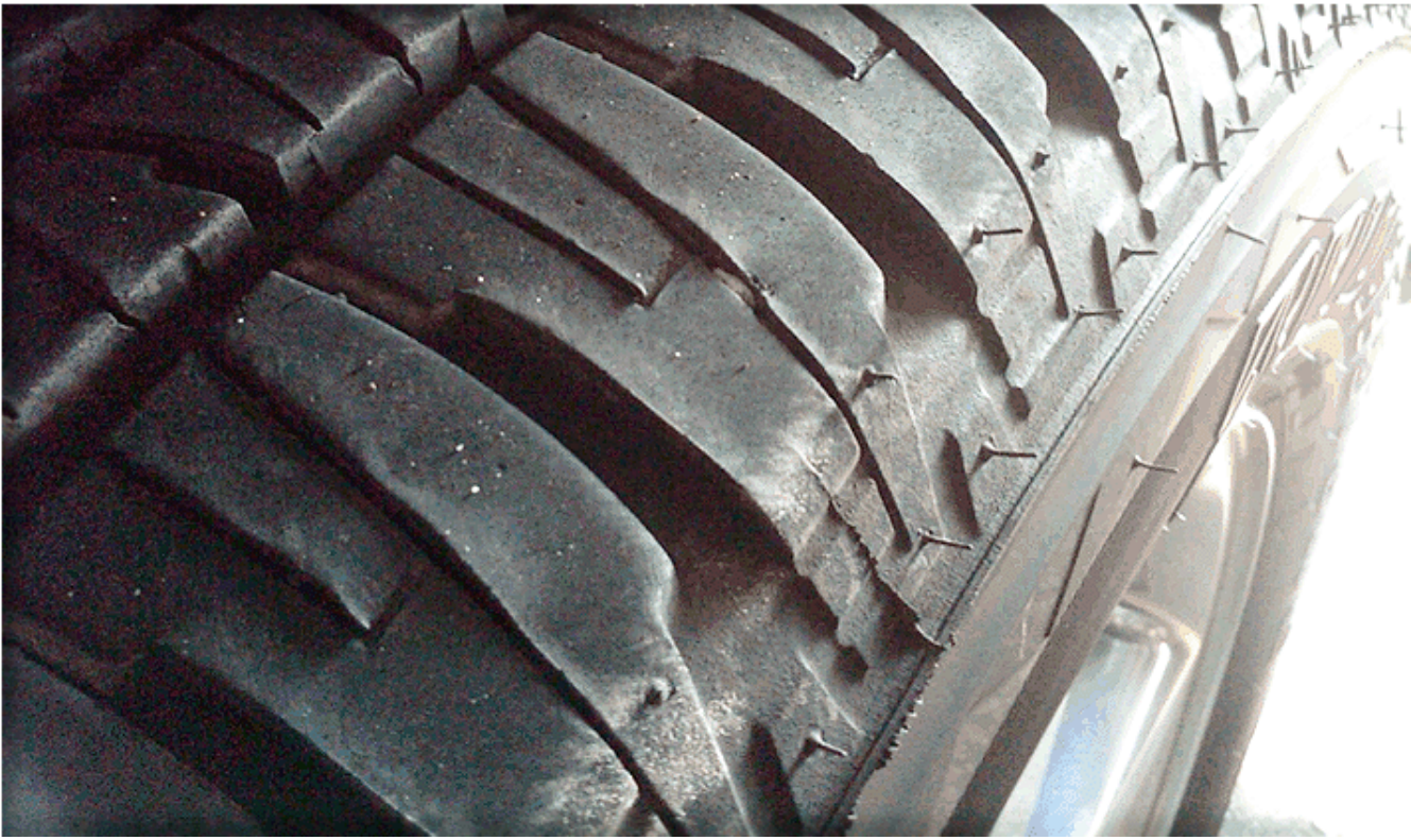
Figure 3: Tire Shoulder View Example 2 - "NORMAL" Tire "Feathering" Wear
