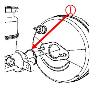
Inspect for the O-ring (1) between the master cylinder and the brake booster before performing any other diagnostics for the low brake pedal or the DTC C027B. Replace the O-ring if missing or damaged.
