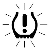
If the TPM indicator appears as a BLINKING yellow lamp for one minute and then stays on solid, diagnostic service is needed.
