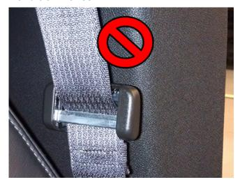
As shown in the graphic above, some customers may comment that the driver or passenger side seat belt is twisted or the latch plate is facing backward on the webbing. Note that the tip of the latch plate is incorrectly positioned outboard of the webbing when stowed.
