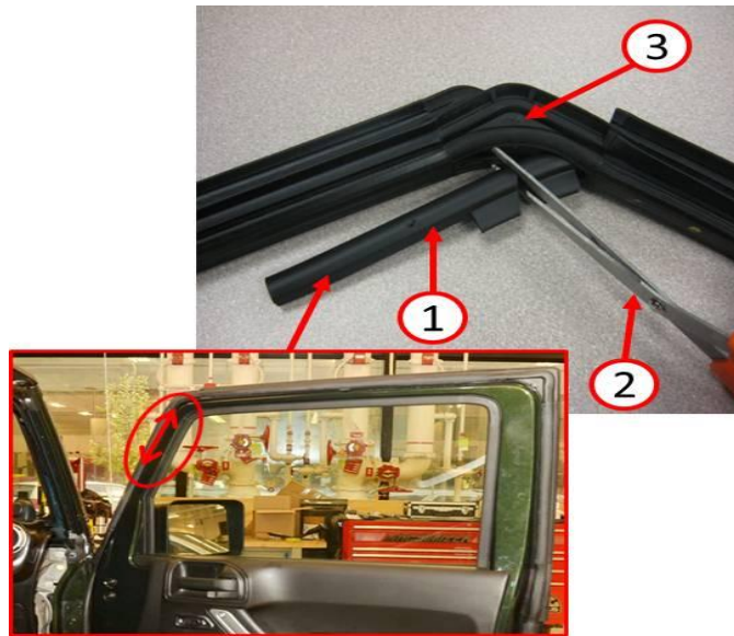
Fig. 12 Door Stuffer Removal
