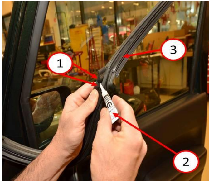
Fig. 14 Door Stuffer Installation
