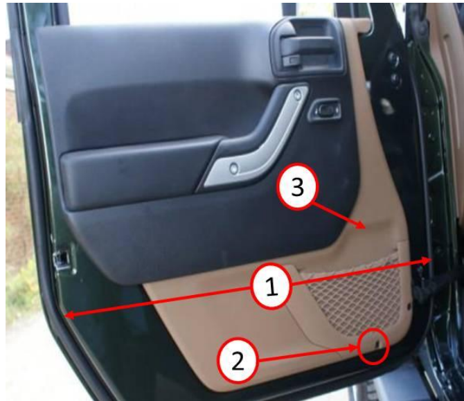
Fig. 2 Door Seal Modification Location
