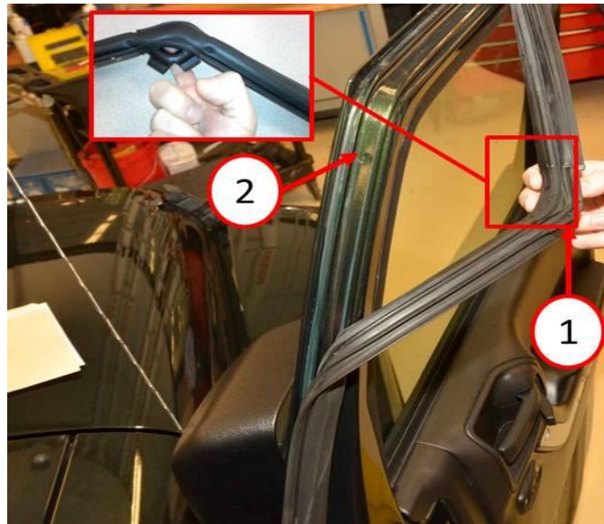
Fig. 10 Door Weatherstrip Removal
