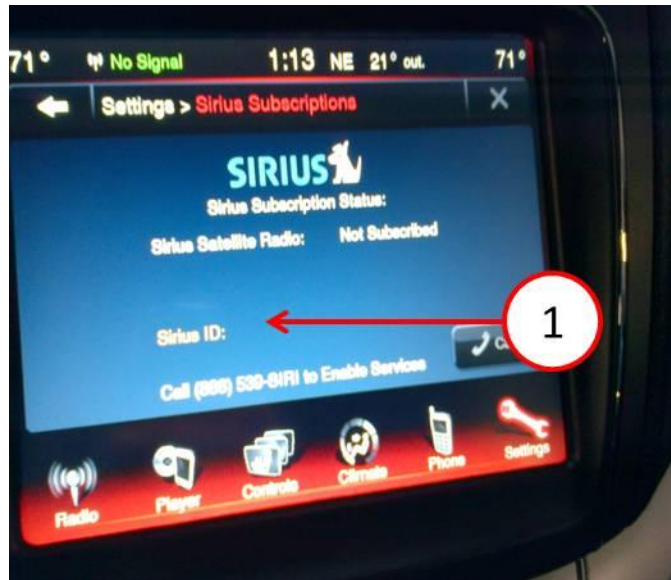
Fig. 1 Sirius ID Number Missing
