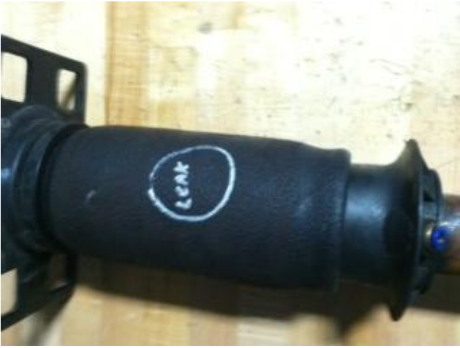
Figure 1 example of marking where air leak was found
