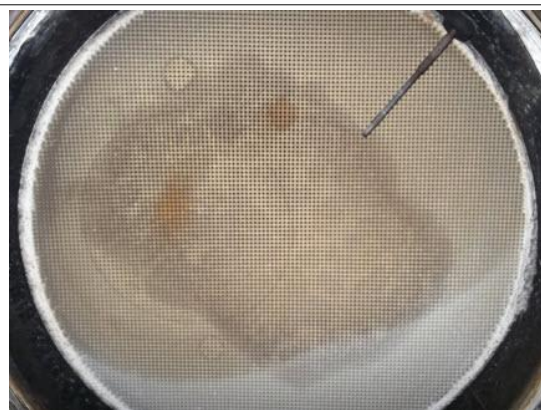
DPF Outlet Coolant Stained - Reusable
