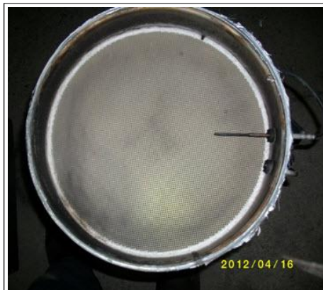
DPF Outlet Normal Operation
