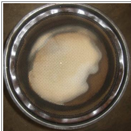
DPF Outlet - Oil Contaminated
