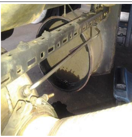
DPF Outlet Coolant - Oil Contaminated
