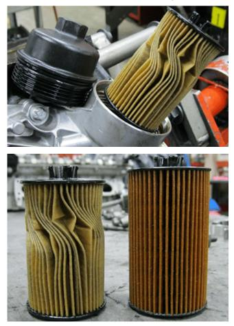
Shown in the illustrations above is an oil filter that was installed improperly, which caused the oil filter to be smashed and cannot close the oil filter drain check valve.
