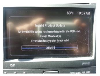
Note: If the following screen above is shown on the screen, the radio already has the latest calibration installed and no further action is required.
