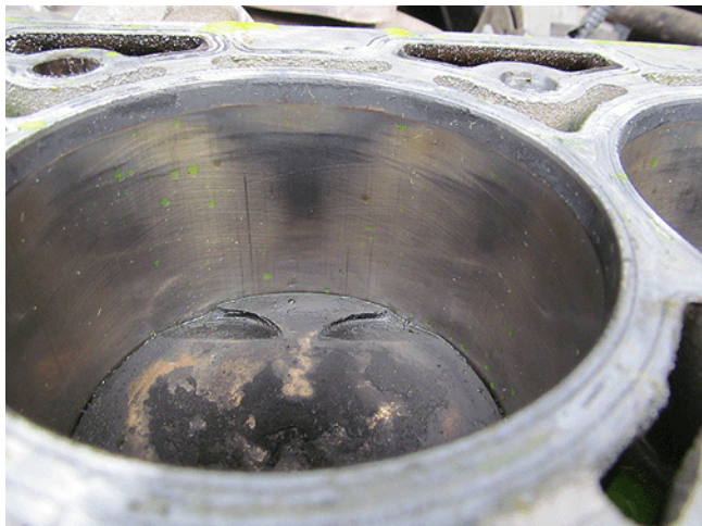
Acceptable Cylinder that Does Not Appear Uniform (Zebra Stripes)
