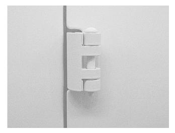
**Note:** A new design for the body side cargo door hinge, shown above, was developed to provide improved resistance to corrosion. New service part kits (which include the body and door side hinges, plates, bolts, stop, pin and instruction sheet) were released for the four hinge locations.
