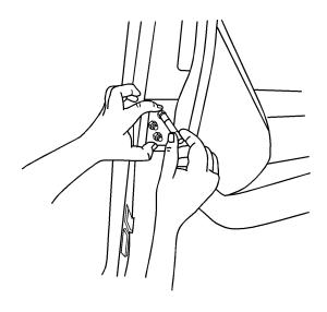
**Important:** For the forward most door (60 door), place the backing plate on the hinge surface and move the plate rearward 4 mm (0.16 in), then mark the three-hole pattern.
