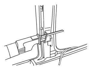
4. Cut the production body side of the door hinge using a reciprocating saw. This is necessary to gain access for drilling out the welds.
