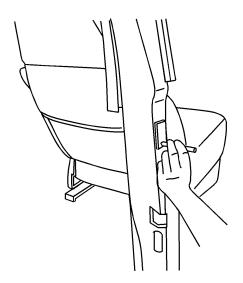
7. Center punch the marked three-hole pattern.
