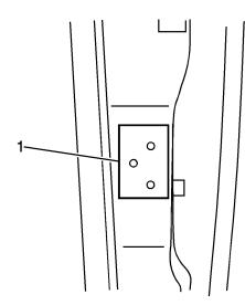
5. Remove any excess sealer surrounding the existing body side hinge, then tape around the periphery of the hinge to mark the hinge location (1).
