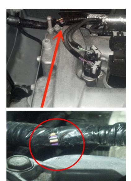
These conditions may be caused by one of the wires (in particular circuits 2500 and 2501) in the engine wiring harness being chafed, cut or damaged due to contact with the right rear corner of the engine or cam/valve cover.
