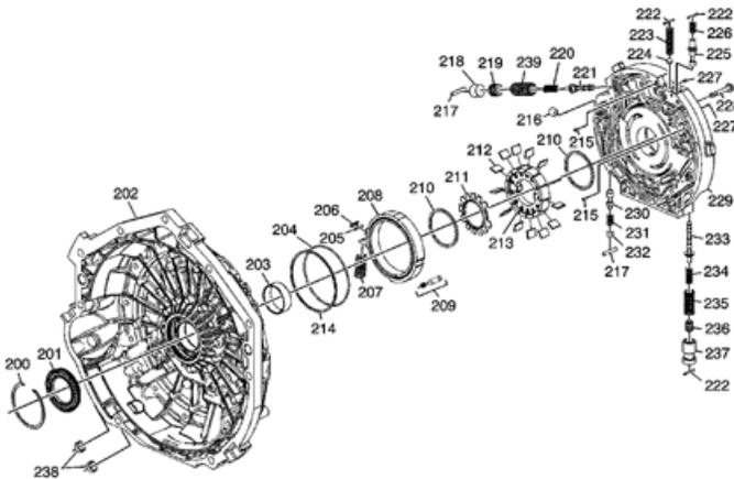
4. Replace the fluid pump cover kit. The cover kit is shown as part number 229 in the picture above.
