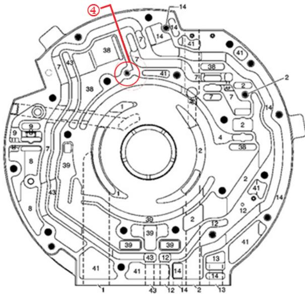
3. Remove and discard the orifice cup plug in the pump cover. The location is shown above (callout #4).
