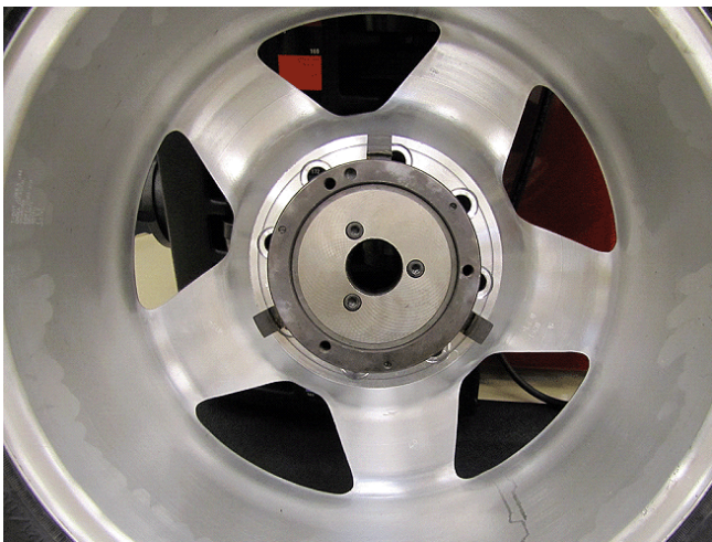
Hunter TruckChuck® Correctly Attached (Front View)
