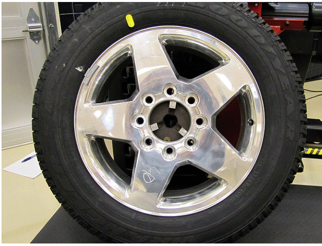
Hunter TruckChuck® Correctly Attached (Close Up)
