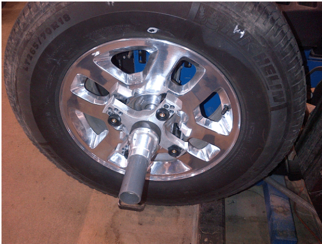
Four Arm Star Mounted to the Front of a Single Wheel Aluminum Rim
