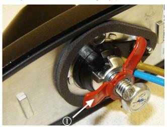
Though difficult to detect evidence of impact damage, upon inspection of the antennas returned in warranty, there is a likelihood this damage occurred during vehicle transportation to dealerships. The result of impact damage is most often to the underside retainer (1), which is found to be bent backward or otherwise damaged and no longer provides proper retention.
