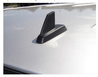
Grasp and physically inspect the XM, cellular mobile phone, and/or OnStar® antenna for looseness and/or damage. If the antenna is mounted securely and exhibits no signs of physical damage, follow regular diagnostic information in SI to address any customer concern.
