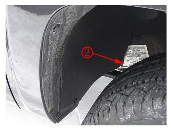
The frame labels are only required during the manufacturing process and can be removed during pre-delivery inspection (PDI). There are two labels on the frame: the left front label (1) visible underneath the driver's door and the right front label (2) visible through the wheelhouse. Use care when removing the labels
