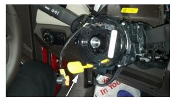
The purpose of this PI is to inform dealership personnel that a SIR locking clip, which will ensure that the SIR coil is not rotated during installation as shown in the illustration above, is available and can be obtained from the Warranty Parts Center (WPC).
