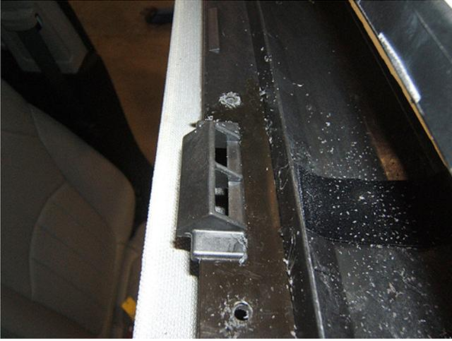
**Important:** When drilling holes, be careful not to drill through the headliner.
