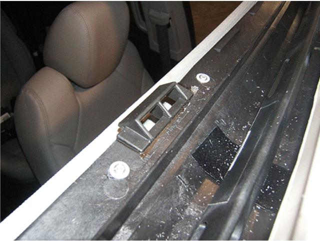
5. Install rivets from the top side to secure the sunroof sunshade striker in place.
