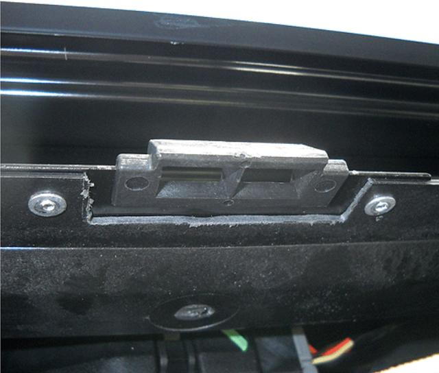
5. Install rivets from the bottom side to secure the sunroof sunshade striker in place.
