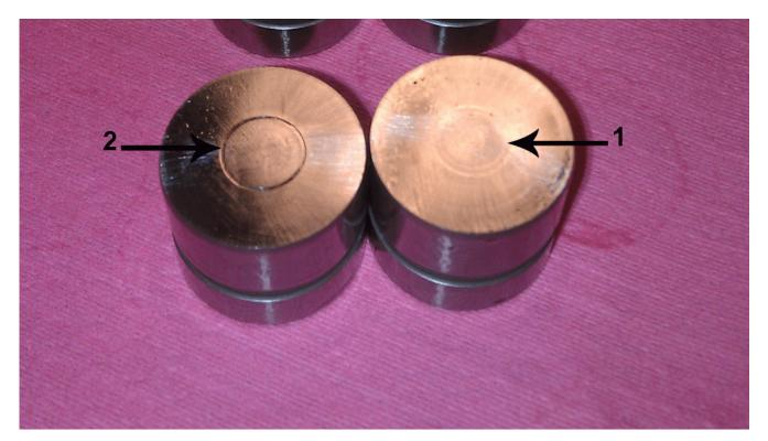
Notice: Refer to this graphic for an example of a normal wear pattern (1) and a circular wear mark (2) on top of the valve lifter body.
