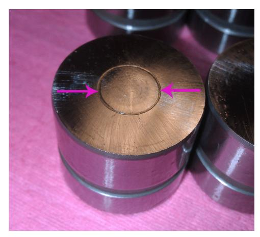
Notice: Refer to this graphic for an example of the circular wear mark on top of the valve lifter body.
