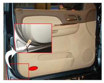
**Note:** The gap is generally 1-2 mm (0.04-0.08 in) as shown by the gauges in the above graphic.
