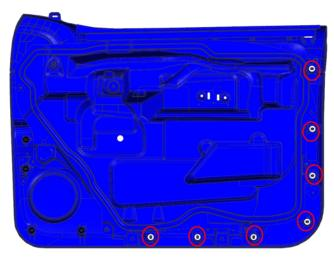
2. Inspect the rear and lower door trim retainers (circled in the graphic above) for damage or improper engagement.
