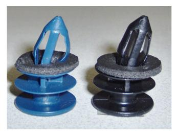
The cause of this condition is most commonly found to be the rear and lower door trim panel retainers, which have been damaged or not properly engaged during installation or R&R of the door trim panel.
