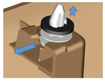
**Tip:** When removing the retainers, a flat-bladed tool is recommended to avoid damaging the molded standing boss on the trim panel. Pull upward on the retainer while sliding it toward the open end of the standing boss.
