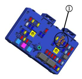
2. Locate the Logistics Fuse (1) and press firmly into the fuse block.
