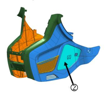
1. With the Key off, remove the IPBEC cover (2) from the passenger foot well inner trim.
