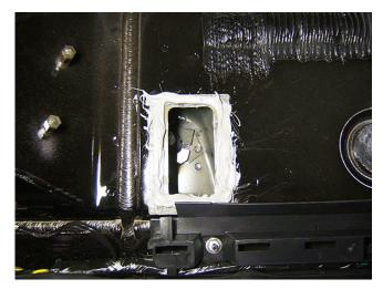
**6.** Coat the perimeter of the access hole with RTV Silicone Sealant, GM P/N 12378521 (in Canada, 88901148) or equivalent, to seal the bare edge of the metal.
