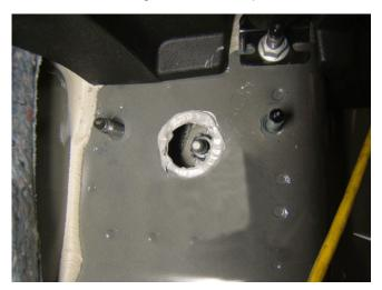
10. Coat the perimeter of the access hole with RTV Silicone Sealant, GM P/N 12378521 (in Canada, 88901148) or equivalent, to seal the bare edge of the metal.
