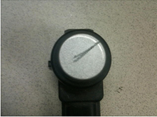
Example #6 – Sensor Detached from Bezel
