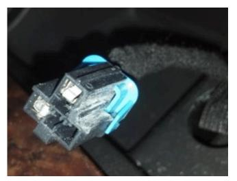
5. Reinstall the CPA retainer to the harness connector.
