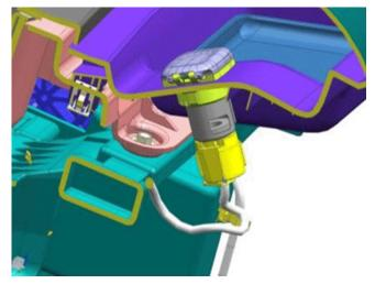
6. Remove the electrical tape and plug the accessory cigarette lighter into the APO harness connector. Ensure the cigarette lighter fully seats on the connector and locks into place.
