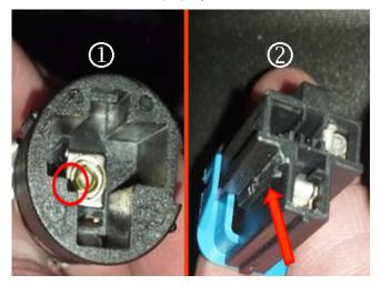
The cause of this condition may be that the engagement slot on the cigarette lighter (1) is on the opposite side as the keyway on the APO harness connector (2). The keyway is obstructing the harness connector from seating properly on the cigarette lighter.
