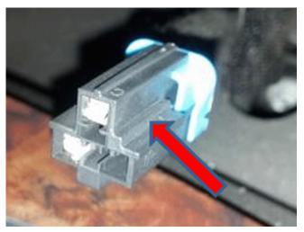
1. Remove the APO plug and inspect the harness connector. Note the location of the plastic key way on the connector, shown by the arrow in the graphic above.
