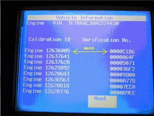
Compare each: **Calibration ID Part Number and Verification No. (Number/CVN)** from your **Tech 2®** photo to the corresponding **Calibration ID Part Number and Verification No. (Number/CVN)** listed in the **TIS2WEB GM Vehicle Calibration Information** screen of **TIS2WEB** to ensure that they are **ALL an EXACT MATCH**.
