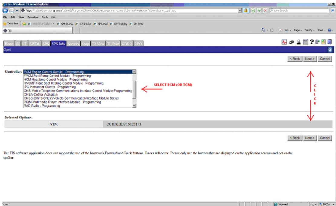
5. Select: **ECM Engine Control Module — Programming** from the Controller dropdown menu and select: **Next**.
