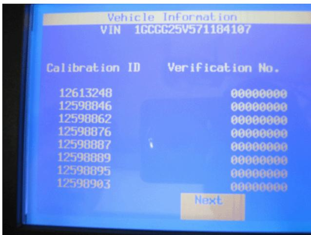
If the Tech 2@ that is being used displays all zeroes for the Verification Numbers as shown, then perform the following steps:
