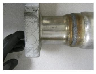
This can be inspected easily by placing a gauge block flush against the flange and inspect for excessive gaps or damage to the flange.
