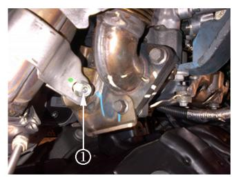
12. Install the mounting bolt (1). If the mounting bracket was removed, align and install the bracket. If the bolt will not line up, bend or shim the bracket until alignment is possible.
