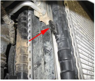
7. Place the grille screen with mounting brackets attached on the new radiator above the existing screen. Align the screen so that the tubes on the radiator are covered and mark the hole locations that will attach to the existing tabs at each end of the radiator.
