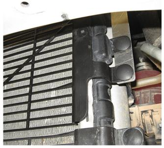
9. Install the grille screen to the new radiator using the retainers.
