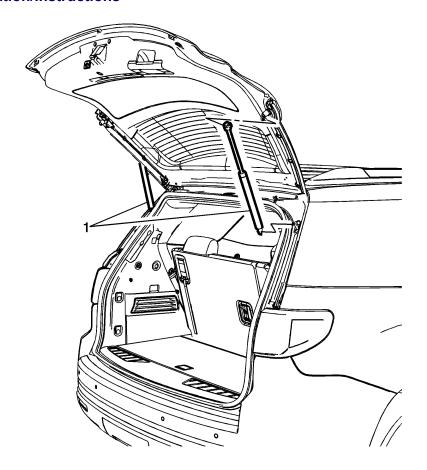
When it is necessary to replace a liftgate strut, install the strut assembly with the strut body end attached to the body side of the vehicle and the rod side attached to the liftgate (1).
