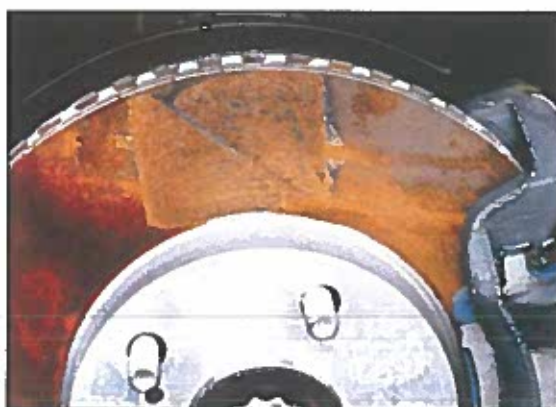
Figure 2. Severe Rust on Rotor (Hard to Remove by Braking)
