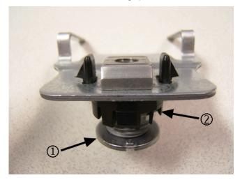
The washer insert (1) of the leveling nut has a reverse thread. Turning it clockwise will increase the gap between the washer and housing (2) and turning it counterclockwise decreases the gap. By design, when the sunroof bolt is installed into the leveling nut, the washer insert will thread downward and open the gap until the washer contacts the topside of the sunroof frame.
