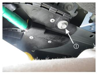
2. Starting on either side, remove the rear sunroof bolt (1) from the module.
