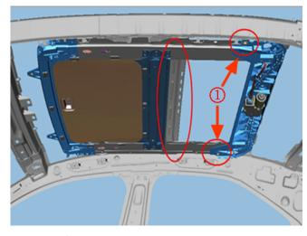
The cause of this condition may be that, during production, the rear of the sunroof module was installed too high when the two rear leveling features (1) were not properly adjusted. When the sunroof glass is open, the distance between the glass and the roof structure #2 bow (shown circled above) is too narrow and contact of the glass to the roof bow may occur.
