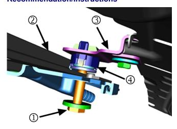
The two rear bolts (1) of the sunroof module (2) thread into a bracket (3), mounted to the roof structure on each side, which contain a unique leveling nut mechanism (4).
