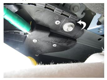
This leveling nut is sandwiched between the bracket and the topside of the sunroof frame, so it is not visible when the sunroof module is installed. A right rear view of the module is shown in the graphic above.
