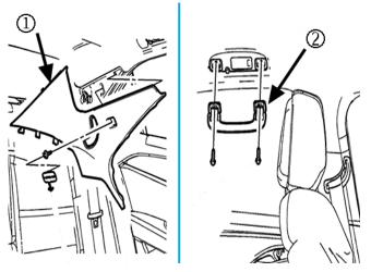
1. Remove the right and left quarter upper trim panels (1), the rear roof rail assist handles (2) and lower the rear of the headliner. Refer to Headlining Trim Panel Replacement (With Sunroof) in SI.
