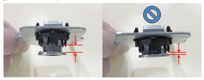
Design intent is to maintain a 5 mm (0.20 in) gap in the leveling nut during installation of the sunroof. The graphics above show the correct/incorrect gap. Verify the condition, then properly adjust the two rear sunroof leveling nuts following the steps below:
