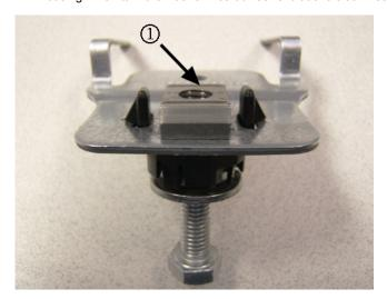
**Note:** To ensure proper adjustment of the washer insert, do not push the bolt hard enough to engage and thread into the nut (1) on the top side of the roof bracket.
