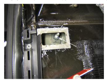
5. Service the cab mounting bolt and nut as required.
