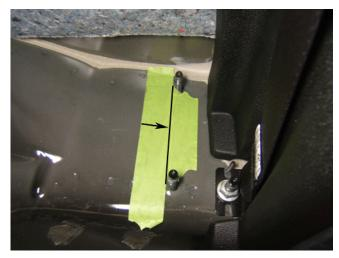
**4.** Using a straight edge, create a line along the inboard side of the seat mounting studs as shown.
