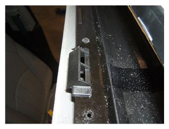
Important: When drilling holes, be careful not to drill through the headliner.
