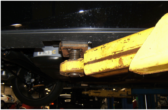
This is a view of the proper front hoist contact lift point.
