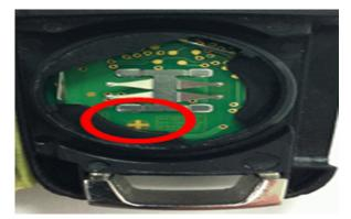
3. If the circuit board has a ± at the 6 o'clock position as shown in the illustration above, replace the key transmitter with the different part number shown below. Refer to key with Integrated Transmitter Replacement and Programming in SI.
