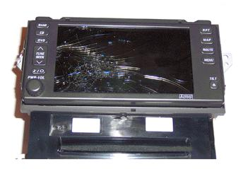
• The illustration above shows a navigation radio with a cracked display window.
