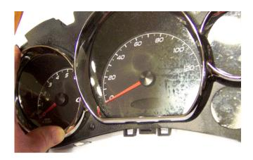
• The illustration above shows an IPC with chemical damage to the lens.
