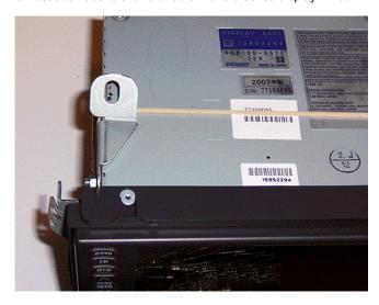
• The illustration above shows a radio with damaged mounting tabs.
