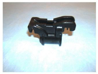
A clip has been made available to eliminate the lateral seat movement. Use the following steps to install the clip to the driver side seat. If the vehicle is equippec with a 6-way adjustable passenger seat, repeat the procedure on the passenger seat.
