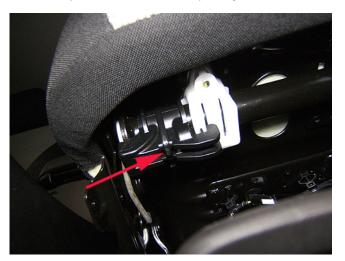
4. Install a nylon wire tie as shown. Trim the excess wire tie material.
