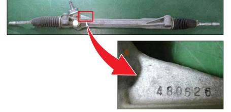
To ensure proper ordering of the service part, confirm the date stamp marking on the steering gear installed in the vehicle and verify if it was produced ON or BEFORE 4/12/2010 by using the legend below:
