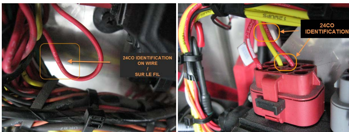
Fig.6 24CO Wire identification on H series (Left) and X series (Right) vehicle.
