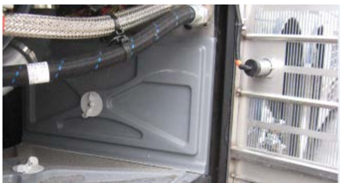
Fig. 2 Electrical compartment cover (X series vehicles)
