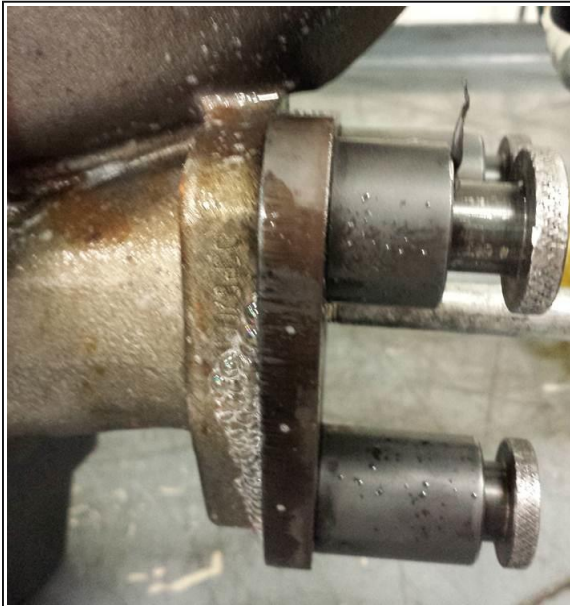
Figure 2: EGR Cooler inlet leak test
