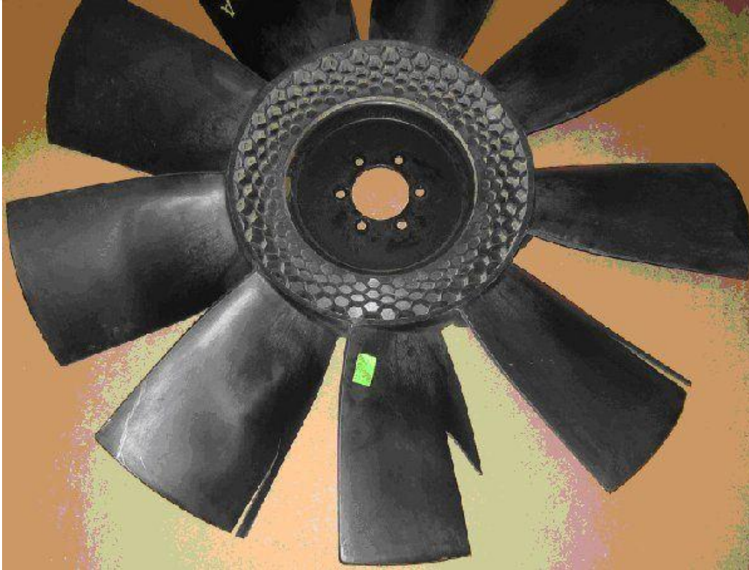
Figure 1. Typical Fan Blade Tip Failures
