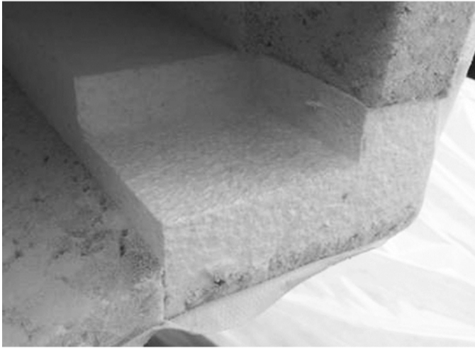
Figure 3. Replaced Seat Back Foam.
