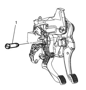
Apply GM Super Lube Part Number 12346241 (in Canada use 10953474) or equivalent around all the gaps on the clutch pedal pin (1) in the illustration above. **Note:** DO NOT remove the clutch pedal pin during the lubrication process.
