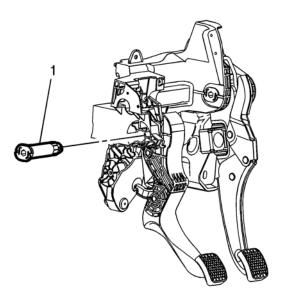
This may be caused from lack of or no lubrication on the clutch pedal pin (1) shown in the illustration above.
